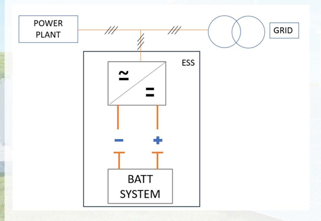
For the Energy Storage System certification integrated in a Power Plan it is necessary to model the full Power Plan including the ESS and simulate the compliance with the Grid Connection applicable standard.
